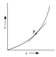
$a=lim\Delta t \rightarrow 0\Delta v\Delta t = dvdt = slope of the tangent at point P$
