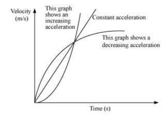
• Area under the *v-t* curve is equal to the displacement of the body.
